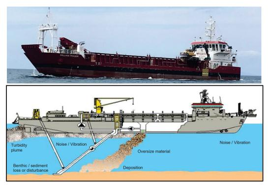
Figure 2. Top: MBL vessel, *William Fraser*, extracting sand from the current Pakiri coastal area. Bottom: Generic illustration of sand extraction and possible impacts, not all of which will be applicable to the current proposal (modified from Bioresearches 2019).
